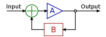
If the feedback is of the same polarity (in-phase) as the input signal it will reinforce (add to) the input signal and cause the output to increase. This is called **positive feedback**.
