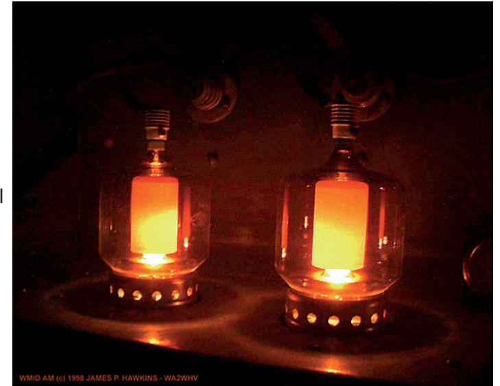
3-500Z transmitting valves undergoing stress testing. If you ever see anodes this colour there is something very wrong! Photo: James Hawkins (Amateur Radio Callsign WA2WHV).
