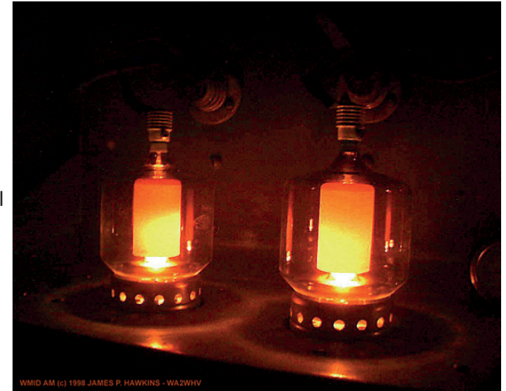
WMID AM (c) 1998 JAMES P. HAWKINS - WA2WHV 3-500Z transmitting valves undergoing stress testing. If you ever see anodes this colour there is something very wrong! Photo: James Hawkins (Amateur Radio Callsign WA2WHV).
